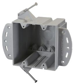
EZ48DN is a 48 cu. in, deep, 2-gang, nail-on, electrical, switch and outlet box for residential or light commercial new construction (new work) electrical installations that also has molded brackets for steel stud mounting. It features 8 wire v-clamps and enhanced angled nails for EZ and more secure installation.
