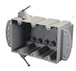
EZ74TN is a 74 cu. in., deep, 3-gang, nail-on switch and outlet box for residential or light commercial new construction (new work) installations with molded brackets for steel or wood stud mounting. It also features 12 contractor preferred wire v-clamps and enhanced angled nails for easy installation.
