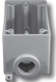
Exposed Boxes Type FDE are designed for use in indoor and outdoor locations where boxes are exposed and subject to environmental conditions. Type FDE is intended for conduit termination with one conduit opening and no outlet. FD boxes are the deepest exposed boxes. They provide space for large devices and additional wiring capacity.
