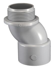
A Meter Offset is used to connect a conduit to a meter box. It is needed to move the path of the conduit away from a wall into the holes in a box or meter box.
