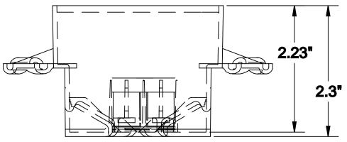
**UL** Listed UL File # R18795 and E98429 2 Hour Ceiling Fire Rated Material is Polycarbonate UL Category Codes CEYY, QBWY and QCMZ 20 Cubic Inches Volume Fixture Weight 50 lbs. Maximum Groung Lug is Included
