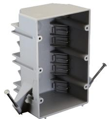
EZ44TN is a 44 cu. in., 3-gang, nail-on, electrical switch and outlet box for residential or light commercial new construction (new work) electrical installations. It features 12 wire clamps and enhanced angled nails for easy installation.
