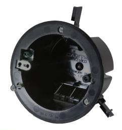
EZ18COG EZ BOX is an 18 cu. in., ceiling box with a ground lug for electrical ceiling applications for (old work) residential or light commercial renovation (old work) projects. The EZ mount flanges, wing tabs and built in wire clamps make installation easy and cost effective. CANTEX ceiling boxes are constructed with durable polycarbonate for added resilience.
