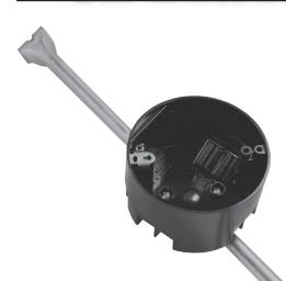
EZ20CHG EZ BOX is a 20 cu. in., new work (new construction) ceiling box with an attached bar hanger for adjustable, support between ceiling joists as well as a ground lug for grounding. EZ20CHG is for residential and light commercial ceiling applications. EZ20CHG features wire clamps and an adjustable bar hanger that adjusts from 14" to 18" for added support and installation options. The EZ20CHL hanger bar adjusts from 18 in. to 24 in.
