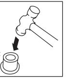
Secure the box to concrete form. Be sure the pour cover is in place to keep concrete out of the box.
