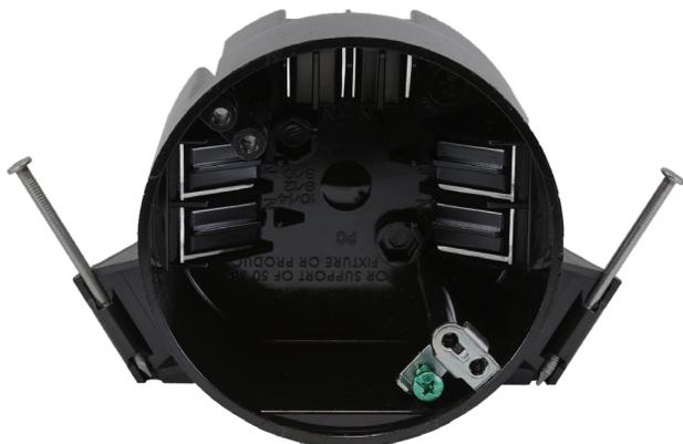
EZ20CNG EZ BOX is a 20 cu. in., new work (new construction) residential ceiling box for residential and light commercial ceiling applications. It features six wire clamps and enhanced angled nails for easy installation and a ground lug for grounding. Attached mounting nails are included.
