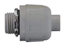
Enviro-Flex® Straight Liquidtight Connector is used to connect Enviro-Flex nonmetallic liquidtight flexible tubing to a box opening or threaded female fitting.
