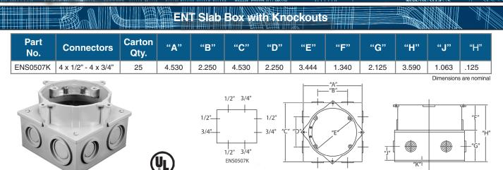
CANTEX ENS0507K is a 55.5 cu. in. ENT Slab Box with 1/2 & 3/4 inch Knockouts designed for use with electrical nonmetallic tubing (ENT) and standard electrical devices and switches in residential and light commercial applications.
