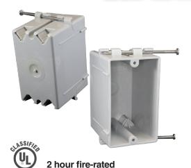
EZ18SN, EZ20SN & EZ23SN are 1-gang, new work switch and outlet boxes with enhanced angled nails that make mounting between studs EZ and more secure. This new construction box features four v-clamps making wiring easier during residential and light commercial installations.
