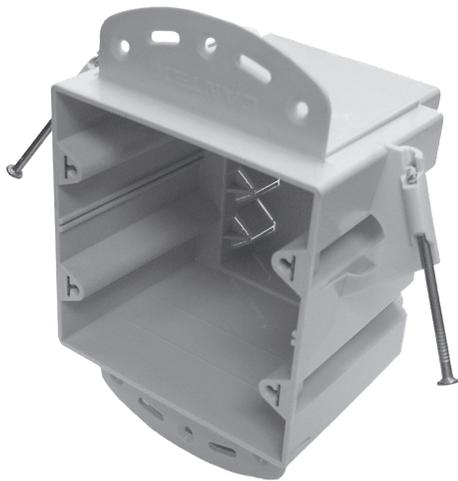
EZ48DNU is a 48 cu. in., deep, 2-gang, nail-on switch and outlet box for residential or light commercial new construction (new work) applications. It features molded brackets for steel stud mounting, v-clamps, and Express Clips® for EZ installation. Express Clips® allow for EZ secure installation of electrical devices. Just align device with mounting holes, push in and turn the screw. It also features 8 contractor preferred wire v-clamps and enhanced angled nails for easy installation.
