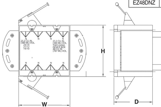
Features 8 V-clamps for EZ & secure wiring
