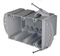
EZ74TNU EZ BOX is a 74 cu. in.,deep 3-gang nail-on electrical switch and outlet box for residential or light commercial new construction (new work) electrical installations. It features molded brackets for steel stud mounting along with v-clamps and an Express Clip® for EZ installation. With Express Clip® there is just one tap, turn and screw for quick secure installation of electrical devices.
