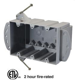
EZ74TNZ is a 74 cu. in., deep, 3-gang switch and outlet box for residential or light commercial new construction (new work) installations with molded brackets for steel stud mounting and screw-nails for EZ installation on aluminum, light to medium grade steel or wood studs. The screw-nail's sharp point, slotted head and threaded body allow for installation with a power screwdriver with no need for pre-drilling.
