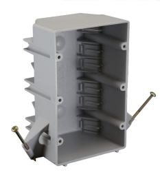
EZ44TNZ is a 44 cu. in., 3-gang electrical switch and outlet box for residential or light commercial electrical installations. It features screw-nails for use on aluminum, light to medium grade steel or wood studs. The sharp point, slotted head and threaded body allow for easy installation using a power screwdriver without having to pre-drill.
