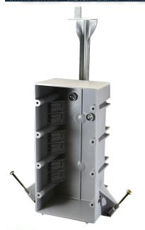
EZ55QNB EZ BOX is a 55 cu. in., 4-gang, nail-on, electrical, switch and outlet box for residential or light commercial new construction (new work) installations. It features an adjustable metal bracket for quick mounting between studs, 12 wire clamps, and enhanced angled nails for EZ installation.
