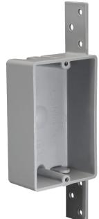
CANTEX EZ08SB is a 1-gang, 8 cubic inch, PVC switch or outlet box that is great for residential and light commercial new construction (new work) applications where a shallow electrical box is needed. It features a molded-on PVC bracket for easy mounting on wood or metal studs.
