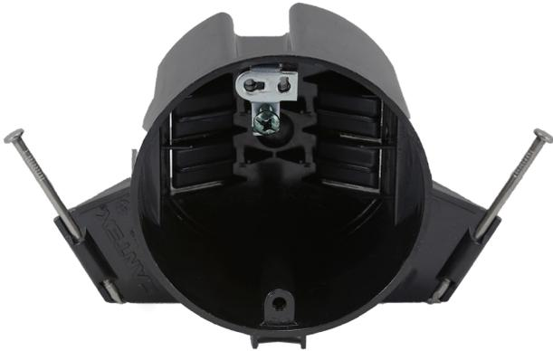
CANTEX EZ18CNG EZ BOX is an 18 cu. in., new work (new construction) residential ceiling box for residential and light commercial ceiling applications. It features six wire clamps and enhanced angled nails for easy installation and a ground lug for grounding. Attached mounting nails are included.
