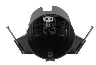
CANTEX EZ18CNG EZ BOX is an 18 cu. in., new work (new construction) residential ceiling box for residential and light commercial ceiling applications. It features six wire clamps and enhanced angled nails for easy installation and a ground lug for grounding. Attached mounting nails are included.
