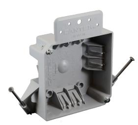
EZ18XN is an 18 cu. in., 4" square, PVC box for residential or light commercial new construction (new work) electrical installations with a molded flange and enhanced angled nails for EZ mounting options. 4" square boxes provide maximum volume for multiple conductors and connectors that often run in two or more directions. Great for walls or ceilings for fixtures, switches or receptacles. CANTEX 4" square boxes are often used with solid PVC blank covers like CANTEX EZXKL.
