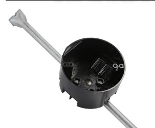
EZ20CH EZ BOX is a 20 cu. in., new work (new construction) ceiling box with an attached bar hanger for adjustable, support between ceiling joists. EZ20CH is for residential and light commercial ceiling applications. EZ20CH features 6 wire clamps and an adjustable bar hanger that adjusts from 14" to 18" for added support and installation options. The EZ20CHL hanger bar adjusts from 18 in. to 24 in.
