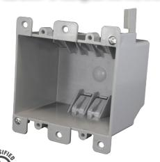
EZ25DO EZ BOX is a 2-Gang, 25 cu. in., renovation application (old work) electrical switch or outlet box for residential or light commercial renovation projects when a 2-gang box is needed. EZ mount flanges, winged swing tabs and built in wire clamps make installation easy and cost effective.
