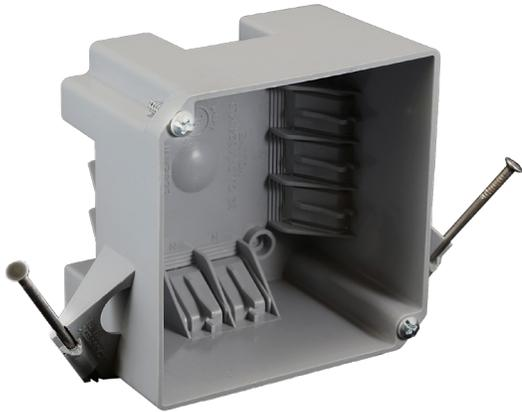
EZ32XN is a 32 cu. in., 4" square, PVC box for residential or light commercial new construction (new work) electrical installations with enhanced angled nails for EZ mounting. 4" square boxes provide maximum volume for multiple conductors and connectors that often run in two or more directions. Great for walls or ceilings for fixtures, switches or receptacles. CANTEX 4" square boxes are often used with solid PVC blank covers likes CANTEX EZXKL.
