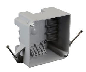
EZ32XN is a 32 cu. in., 4" square, PVC box for residential or light commercial new construction (new work) electrical installations with enhanced angled nails for EZ mounting. 4" square boxes provide maximum volume for multiple conductors and connectors that often run in two or more directions. Great for walls or ceilings for fixtures, switches or receptacles. CANTEX 4" square boxes are often used with solid PVC blank covers likes CANTEX EZXKL.
