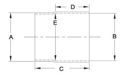
CANTEX 5163551 is a 4 in.CAO Type C Bell to IPS Plain Adapter is designed to transition CAO Type C conduit to IPS trade size conduit.
