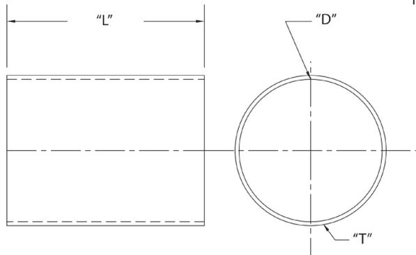
CANTEX 6161652 is a 4 in. CAO Type C Coupling with no center stop used to join lengths of CAO conduit pipe together with two solvent weld socket ends.
