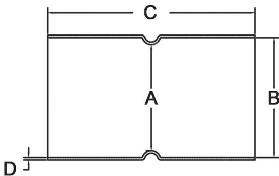
CANTEX 6161632 is a 4 in. CAO Type C Coupling with center stop used to join lengths of CAO conduit pipe together with two solvent weld socket ends. The center stop helps determine the proper depth of the connection.
