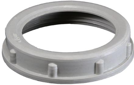
Insulating Bushings are used to terminate threaded conduit or connectors to a box to protect wires from sharp edges and abrasions during pull.
