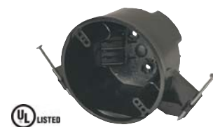
25 CUBIC INCH CEILING BOX Suitable for fixture support only 50 lbs. maximum
