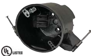
25 CUBIC INCH CEILING BOX WITH GROUND LUG Suitable for fixture support only 50 lbs. maximum
