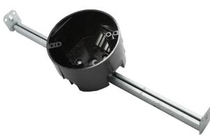
EZ20CHL EZ BOX is a 20 cu. in., new work (new construction) ceiling box with an attached bar hanger for adjustable, support between ceiling joists. EZ20CHL is for residential and light commercial ceiling applications. EZ20CHL features 6 wire clamps and an adjustable bar hanger that adjusts from 14" to 24" for added support and installation options.
