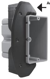
Adjusts from 0 to 1 3/4 inches. EZ22SBZ-ADJ EZ BOX is the CANTEX 1-gang, adjustable, 22 cu. in., new work, electrical switch & outlet box with an adjustable bracket that adjusts to various drywall thicknesses and wall finishes. It is a perfect solution when a wall covering has already been installed. It is great for construction and retrofit applications. It is easy to mount to standard wood or metal studs.
